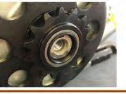
Install the grease trap with the sprocket side facing the sprocket. The sprocket side is stamped "SPROCKET SIDE".
