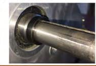
STEP 8 Install the bearing race.
