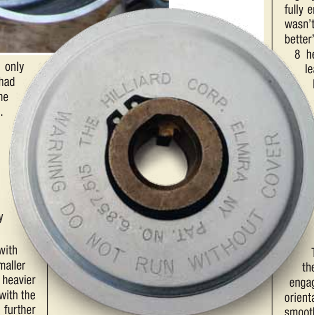
Below: The shield on the clutch keeps the dirt and grime out of the clutch for maximum performance and longevity.
