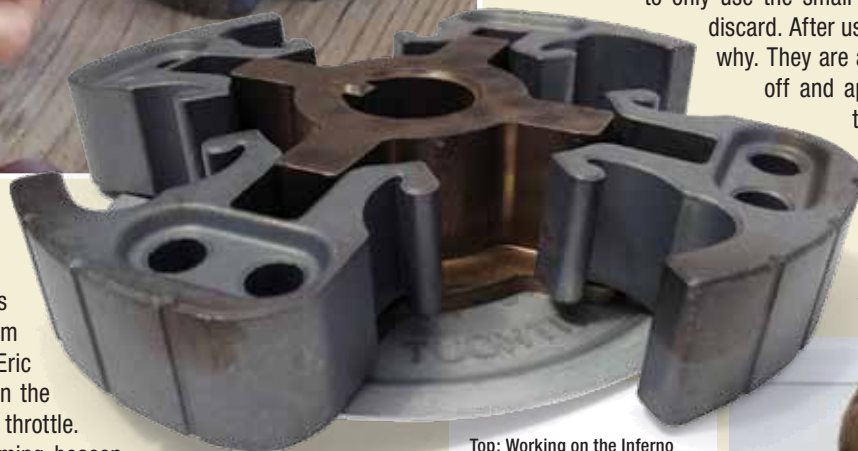
Top: Working on the Inferno Clutch is easy. Snap ring pliers is the only tool needed to make changes.
