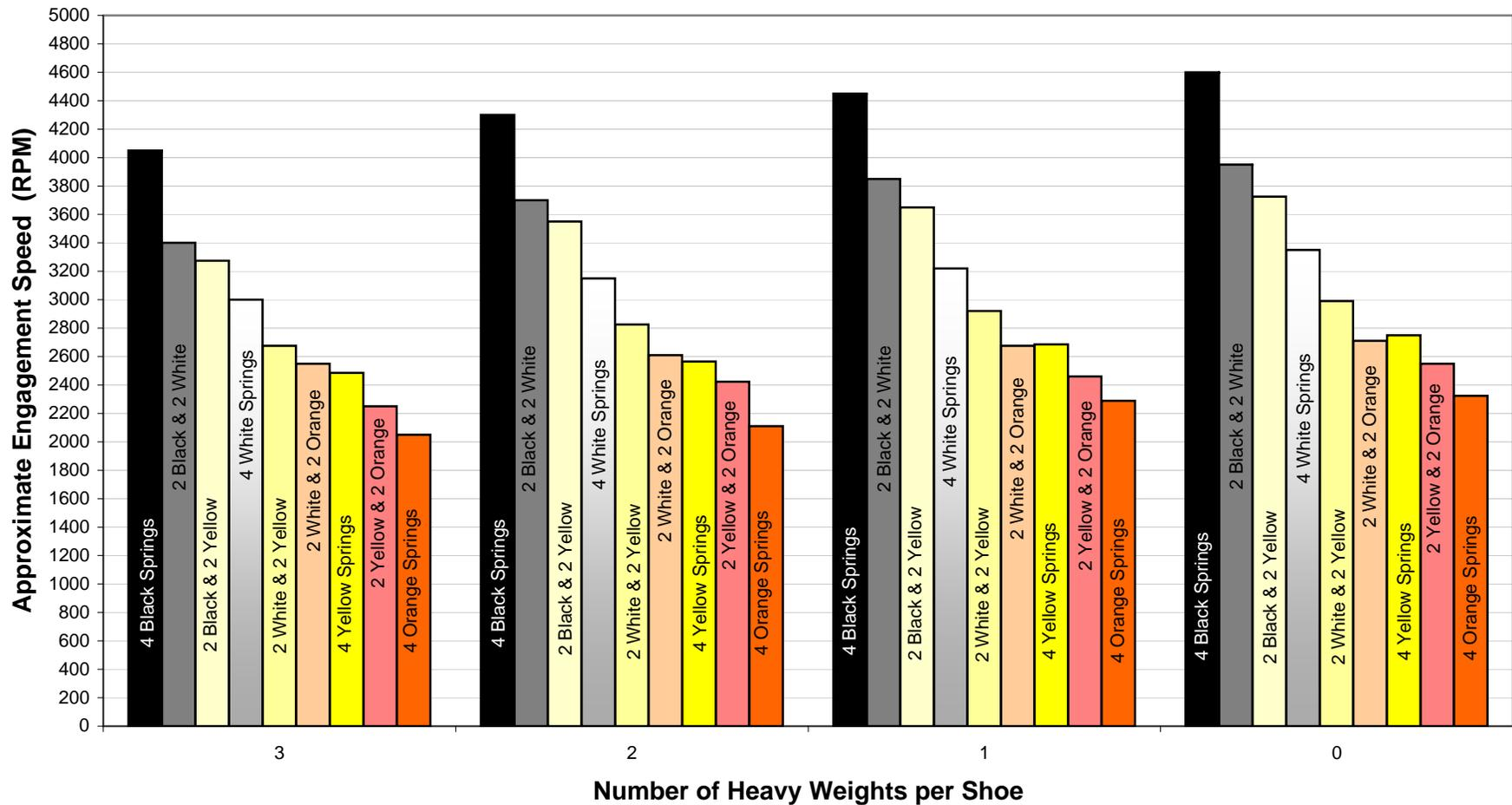
\* Engagement speed is defined as the speed at which the shoes first touch the drum. (NOT LOCK UP SPEED)
