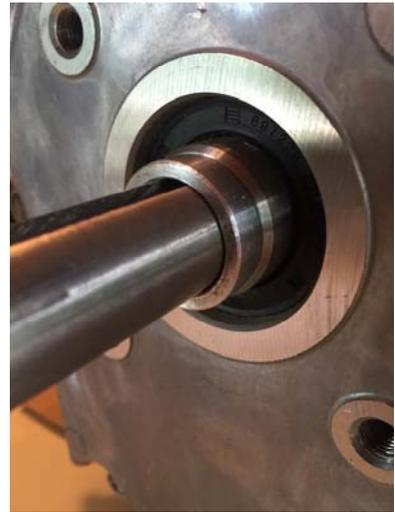
Install the  $\frac{3}{4}$ " x 1  $\frac{1}{16}$ " OD x .04" thick steel washer against the crankshaft spacer.
