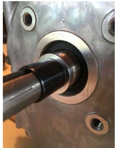
**Lubricate the needle bearing with a high temperature bearing grease and install the needle bearing.**
