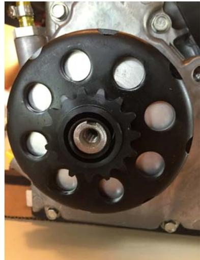
**Lubricate the needle bearing with a high temperature bearing grease and install.**
