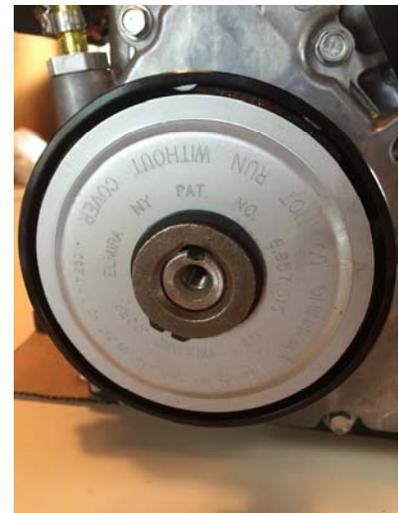
**Properly spaced clutch. The clutch will be clamped tight on the crankshaft to minimize fretting of keyway and potential damage to the integral keys.**
