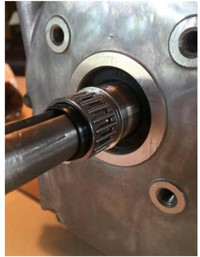
**Install the drum/sprocket assembly. The sprocket will slide over the needle bearing easier if you rotate the drum while installing.**
