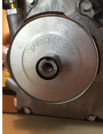
**Install the drum/sprocket assembly.**
