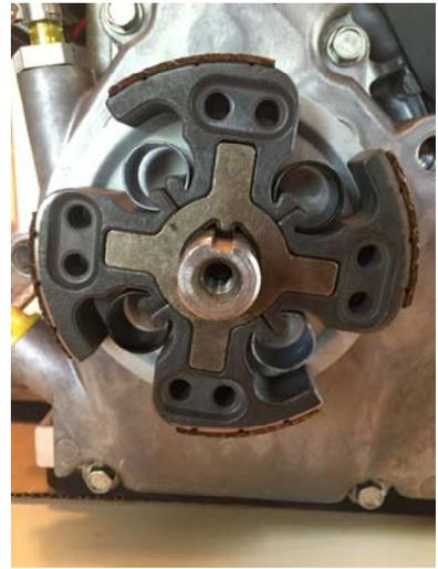
**Install the spring/shoe retaining washer.**
