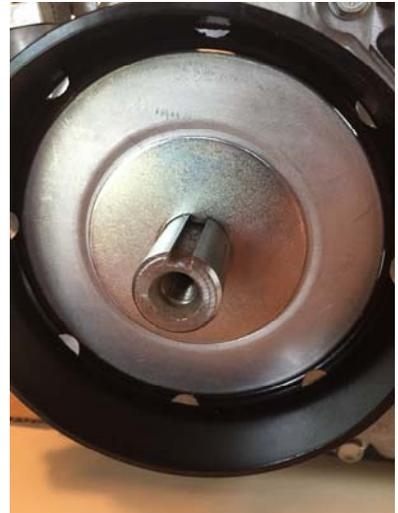
**It is recommended to install the clutch in leading orientation. refer to the pictures for correct positioning of the shoes. These illustrations apply only when mounting the sprocket inboard. Tuning information listed in the back of the instructions.**
